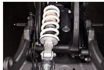
Horizontal Back-link rear suspension
