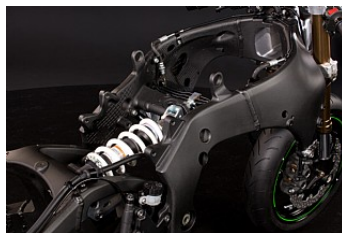
Aluminium Twin-spar frame
