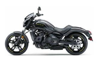
Single 300mm disc with twin-piston caliper
